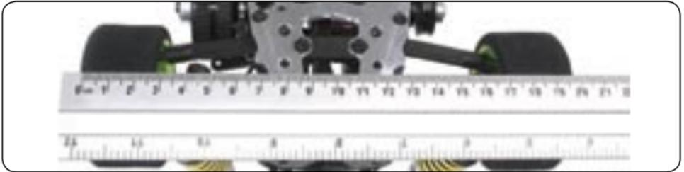
Track-width affects the car's handling and steering response. Front track width can be adjusted between 198–200mm. Rear track width can be adjusted between 196–200mm.
