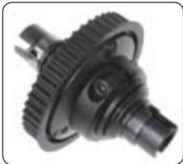
The rear differential shares the same design as the front differential. It is designed to allow separate adjustment of pulley slip and differential action. The differential action is easily adjusted with a single external screw.
