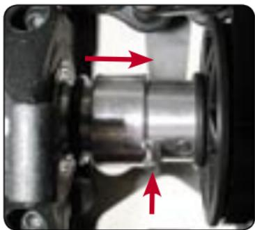
The 710 front one-way axle can be very quickly converted into a solid front axle by inserting two steel pins through the front axle and both drive adapters. An alu. bushing holds the pins in place.
