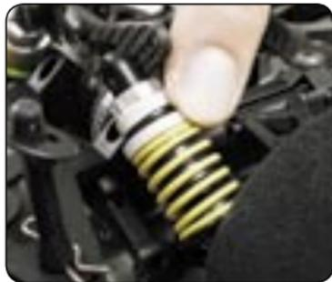
Make sure you change the shock preload on both front shocks equally.
