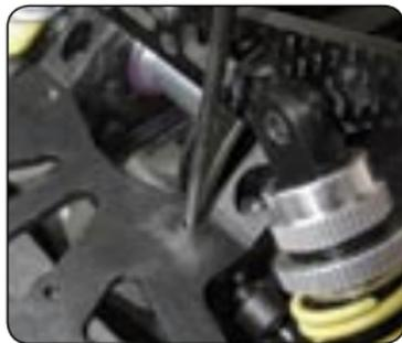
Adjust front downstops by turning the front downstop setscrews in or out. Turn the front setscrews IN to increase the front downstop value. Turn the front setscrews OUT to decrease the front downstop value. Make sure you adjust front downstops so they are equal on both left and right sides.
