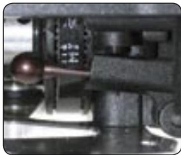
In general, more suspension travel (lower downstop value) makes the car more responsive but less stable; it is also typically better on a bumpy track or on a track with slow corners. Less suspension travel (higher downstop value) makes the car more stable; it is typically better on a smooth track.
