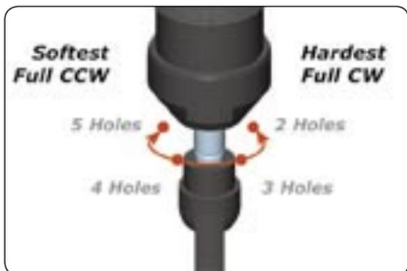
Serpent shocks can be assembled with non-adjustable or adjustable pistons. The non-adjustable pistons use a 1-piece piston with 2, 3, or 4 holes in it. The Serpent adjustable pistons use a unique 2-piece piston assembly that can be easily adjusted to align 2, 3, 4, or 5 holes.
