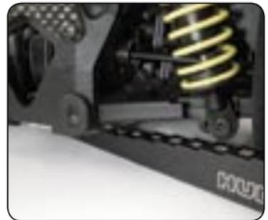
Measure and adjust ride height with the car ready-to-run but without the body. Use the shock preload collars to raise and lower the ride height.
