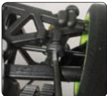
The rear anti-roll bar is adjusted in two ways. There are two positions on the lower arms where the linkages connect; the inside position is the softer setting, and the outside point is the stiffer setting.
